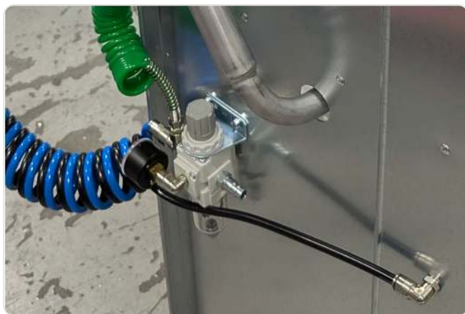
Outside (steps 1–2): black hose through the wall, green hose to compressed air. Red marking = coupling.
